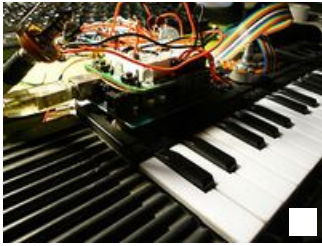
A synthesizer powered by an Arduino
